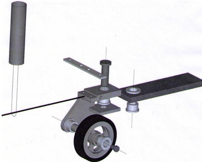
Your tail wheel has been manufactured from quality components and designed to last hundreds of hours under high vibration and adverse weather conditions. Hardware and attachment points have been provided for two steering methods. We highly recommend using locktite on all fasteners. We also recommend you steer the wheel with .062 music wire extending to a hoop in the back of the rudder. Be sure to
