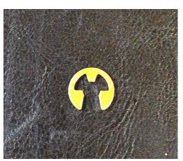
is a picture of a typical "C" clip. Note the three prongs or protrusions in the inside of the clip. It is imperative that all three of these be firmly seated into the groove in the axle. It is also important that the axle groove not have any accumulated grunge packed into it. Since these photos were taken we have improved the security of the retention by making the groove in the axle twice as wide so two clips can be installed in each groove.
