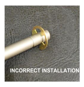
The simplest way to be sure your clips are installed correctly is to be sure the outside diameter of the "C" clip is perfectly centered inside the wheel hub
